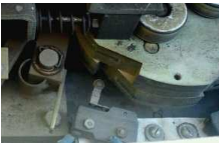
Earlier design employing hinged roller microswitches – Ratchet Activated
